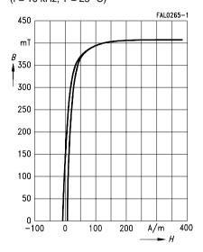
DC magnetic bias (measured on RM cores, typical values) ( $\hat{B} \le 0.25$  mT, f = 10 kHz, T = 25 °C)
