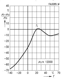
Initial permeability  $\mu_i$  versus temperature (measured on R9.5 toroids,  $\hat{B} \le 0.25$  mT)
