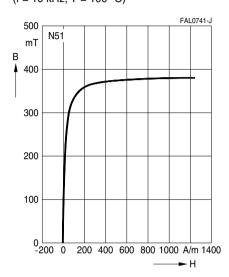
DC magnetic bias measured on E cores ( $\hat{B} \le 0.25$  mT, f = 10 kHz, T = 25 °C)
