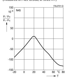
Initial permeability  $\mu_i$  versus temperature (measured on R29 toroids,  $\hat{B} \le 0.25$  mT)
